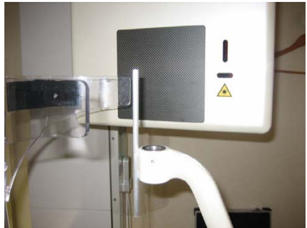
Fig. 2 First step in measuring the MTF. An aluminum pipe was set on the Accuitomo F8 at a slight inclination to the vertical
