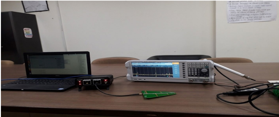
Fig. 1 Measurement set up for recording signal strength
