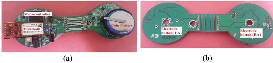
Fig. 4 Wireless ECG assembled PCB a Top view b Bottom view
