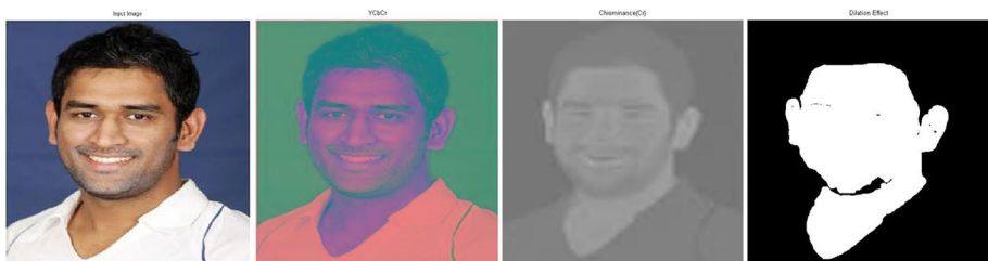
Fig. 4 Face-Region Localization using Skin based Modelling [10] (i) Source RGB Image (ii) Converted YCbCr Image (iii) Extracted Chrominance (Cr) Image (iv) Skin Segmented Image
