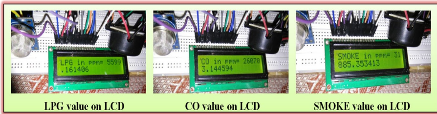
Fig. 6 LCD displaying ppm value of LPG, CO and Smoke
