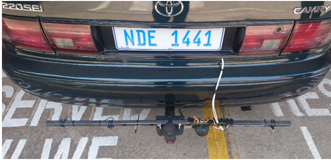
Fig. 18 Distance sensors and GPS module on vehicle
