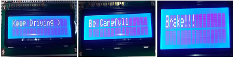
Fig. 8 Warning messages display on LCD at threshold levels
