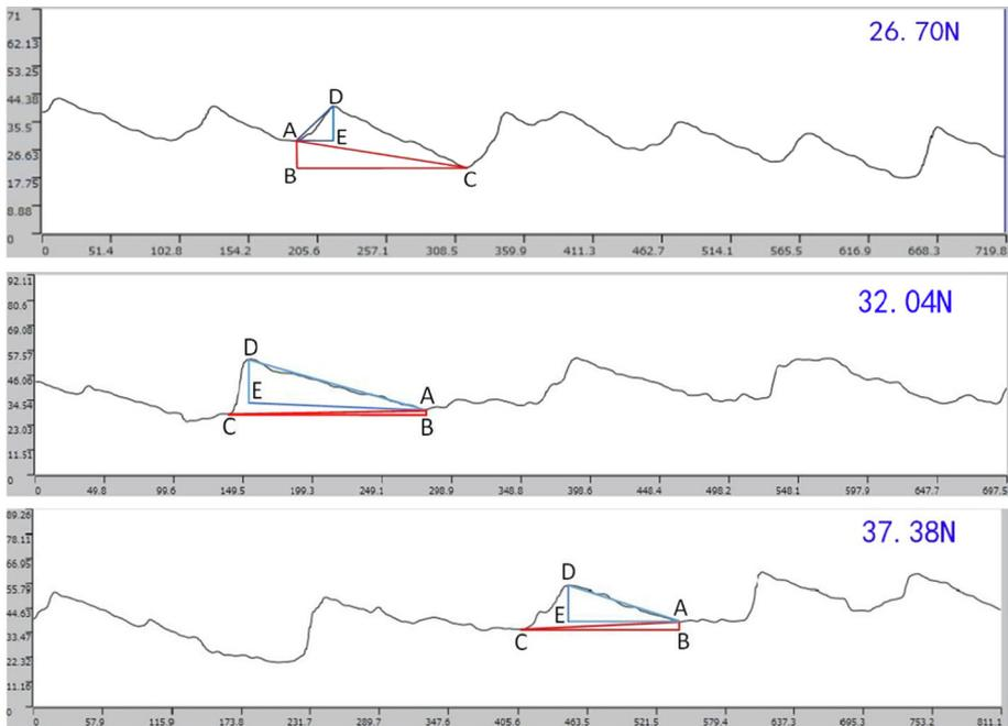
**Fig. 6** The abrasion surface contour curves under different loads
