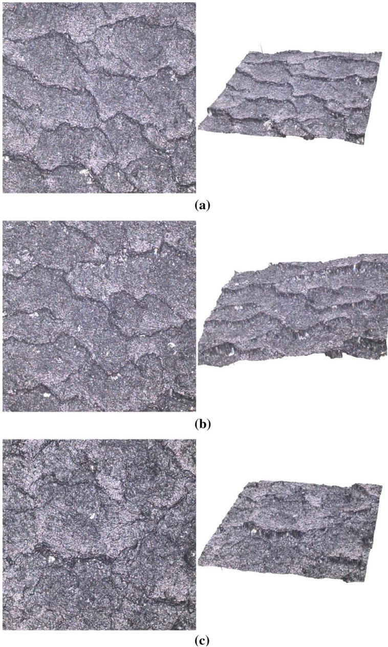
**Fig. 1** 2D and 3D microscope images of abrasion surface at different temperatures
