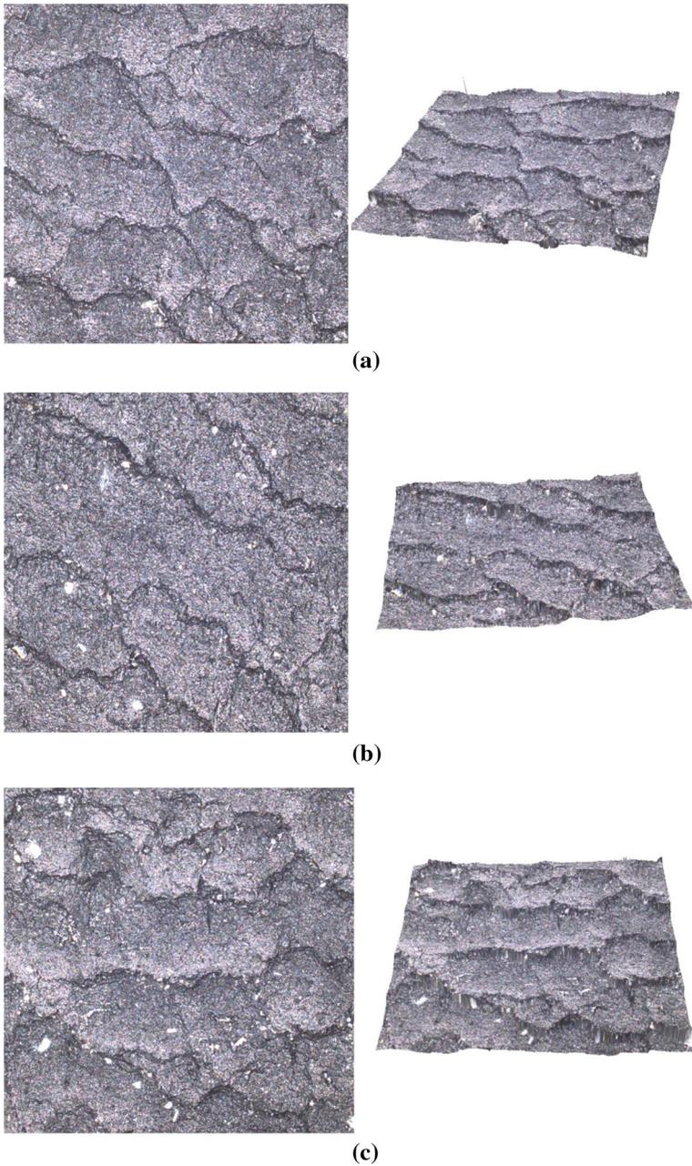
**Fig. 3** 2D and 3D microscope images of abrasion surfaces under different loads. **a** 26.70 N, **b** 32.04 N and **c** 37.38 N
