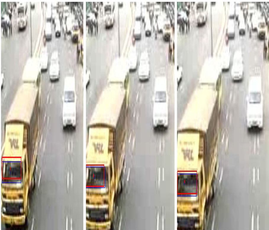
Fig. 8 Tracking of real time vehicle in Frame 19, 20 and 21 of Input video
