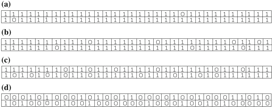
Fig. 8 The packet maps in the memory of each RM after a relays its batch fragment. a The packet map in the memory of b after a relays its batch fragment, b the packet map in the memory of c after a relays its batch fragment, c the packet map in the memory of d after a relays its batch fragment, d the packet map in the memory of e after a relays its batch fragment
