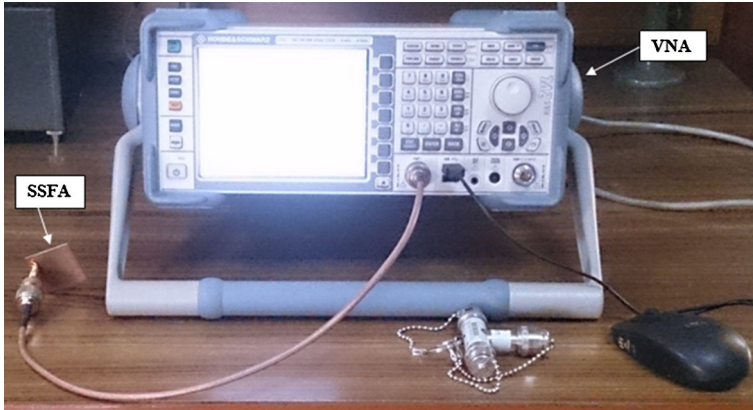
Fig. 11 Rohde & Schwarz ZVL Vector Network Analyzer for testing SSFA
