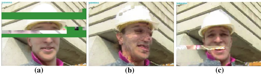
Fig. 2 Equal packet loss in different video frame type. a I-frame packet loss, b P-frame packet loss, c B-frame packet loss
