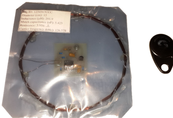
Fig. 14 The relative size comparison of an off the shelf and the designed RFID tag
