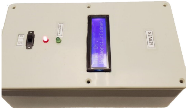
Fig. 16 Data coordinator/Access point device
