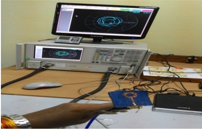
Fig. 10 Proposed antenna while measuring input impedance on vector network analyser in IIT Kanpur lab
