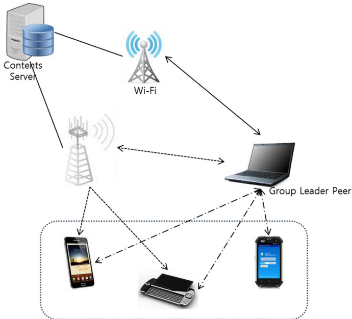
Fig. 2 Network structure of mobile streaming
