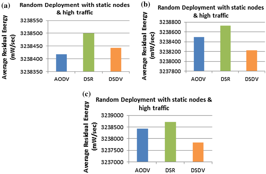
Fig. 10 Average residual energy for scenario 1. a Network of 25 nodes. b Network of 50 nodes. c Network of 75 nodes
