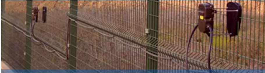
Fig. 1 Over the fence alarm network application of WSN, a simulation model, b field application (Courtesy of Genetlab Inc.)
