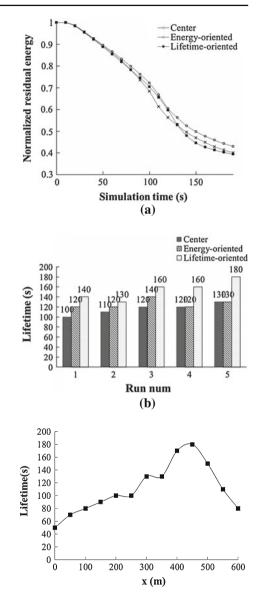
**Fig. 5** The network lifetime of different positions in multi-hop case (y = 300 m) Eq. (41)
