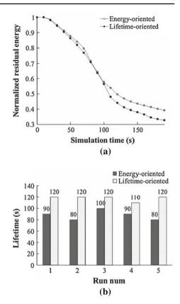
sume more energy to finish the communication. Figure 3b shows the network lifetime of the two placement strategies. Compared with the energy-oriented strategy, the lifetime-oriented strategy prolong the lifetime by more than 20% in each run. The improvement of lifetime performance is attributed to the high node density in  $S_i$ .
