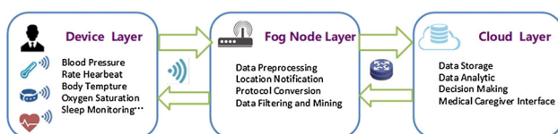
Fig. 2 Proposed fog-driven IoT personal health monitoring system
