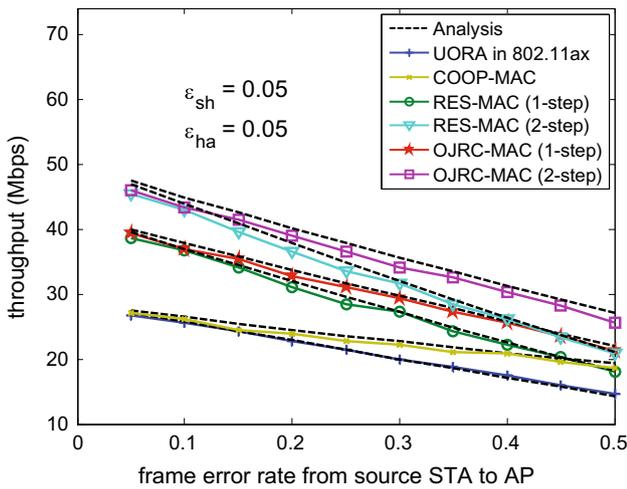
**Fig. 15** Throughput with different frame error rates from the source STA to AP (4 RUs)
