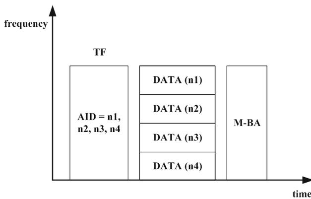
Fig. 2 TF-based UL MU transmission
