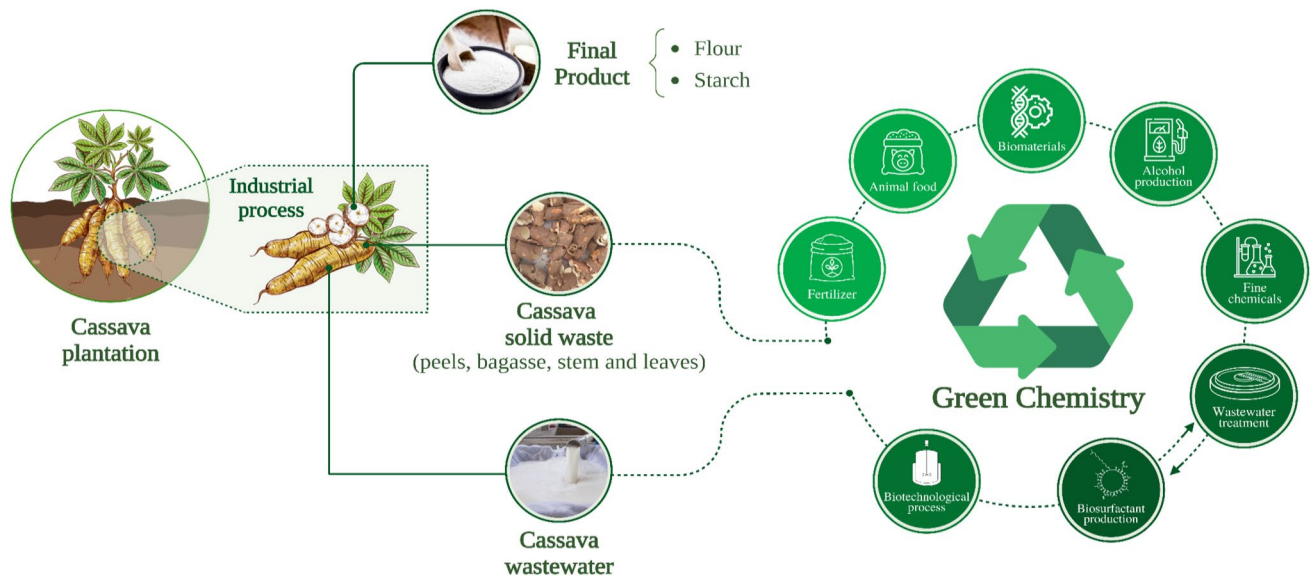
Fig. 1 General flowchart of cassava processing and ecofriendly potential of its residues in the concept of biorefinery
