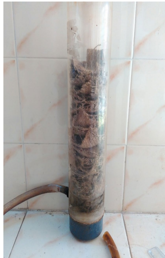
Fig. 2 Packed-bed reactor column with single substrate (JFM)
