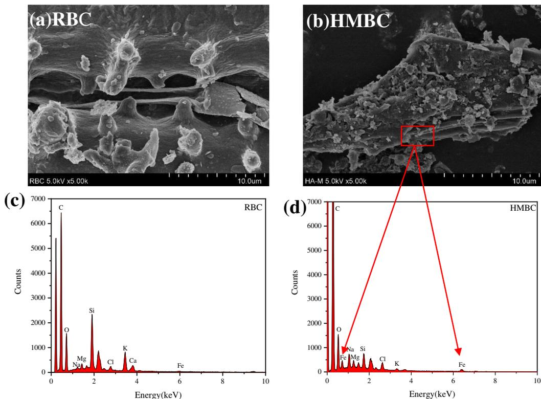
**Fig. 3** SEM images of (a) RBC, (b) HMBC, (c) EDS image of RBC and (d) EDS image of HMBC
