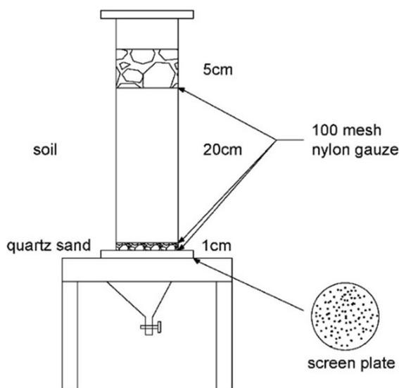
**Fig. 1** Schematic diagram of soil column
