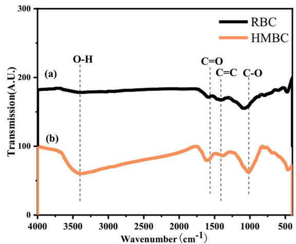
Fig. 2 Characterization of (a) RBC, (b) HMBC by FTIR
