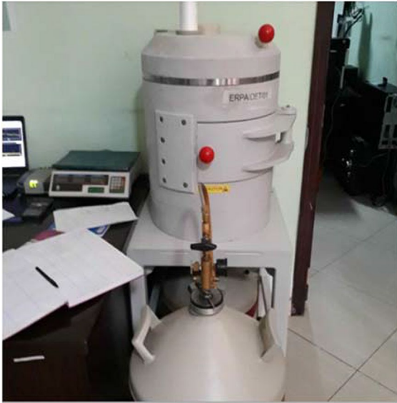
Fig. 2 HPGe detector system produced by the American company Ortec
