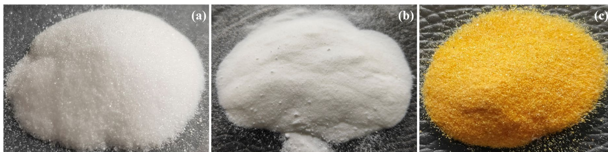
Fig. 2 Physical appearance of a free silica gel ( \text{SiO}_2 ), b \text{SiNH}_2 , c \text{SiNP-L}_3
