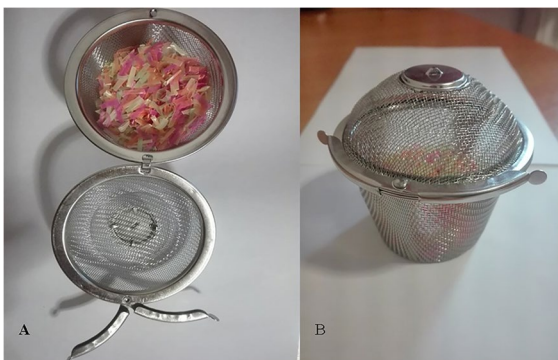
Fig. 1 Plastic colonizer design a open plastic colonizers made from commercial stainless-steel filter filled with 3 g of cut plastic straw. b Closed plastic colonizer filled with plastic straw pieces (< 5 mm)
