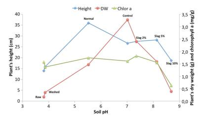
DW). Even though an enhancement in biomass of 1.59 g–DW was obtained when steel slag treatment was increase to 5%, it was evident that a negative trend appeared under alkaline soil conditions (pH over 7.5). For slag 10% treatment, the declining trend went even further whit a weight of 0.40 g–DW shown.
