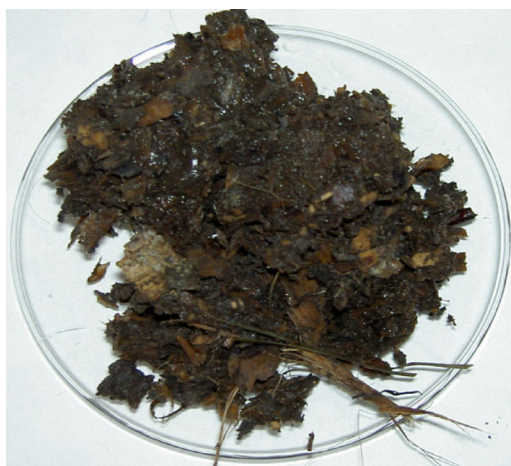
(A) Rural sewage sludge composted with sawdust
