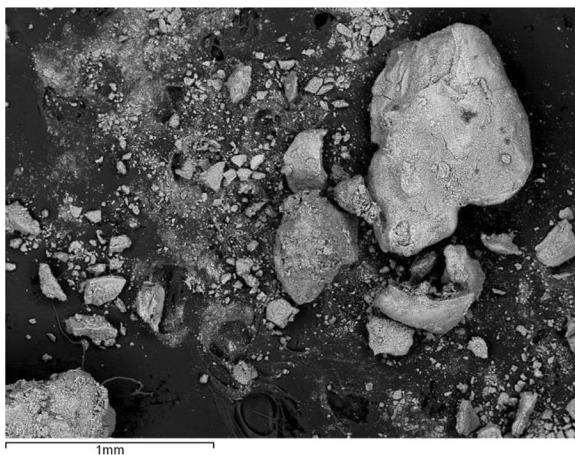
Fig. 4 FESEM surface morphology of white precipitate sample
