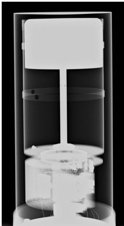
Fig. 2 Radiograph of the detector crystal used in experimental measurements and Monte Carlo simulations
