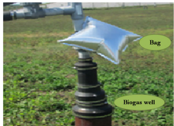
Fig. 3 Sampling the biogas from the biogas well
