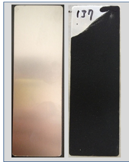
Fig. 2 Aluminum electrode before and after AC coating
