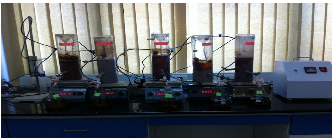
Fig. 1 Reactor set up for with controlled aeration, agitation and temperature for semi-continuous reactor study
