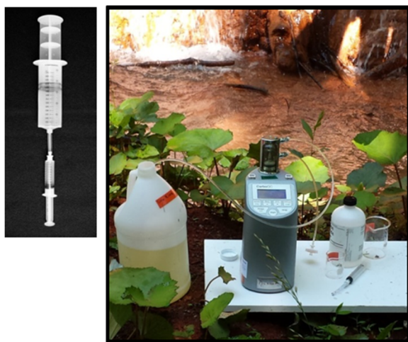
Fig. 2 Connecting the small buffer-containing syringe with the 140-mL sample-containing syringe; carbonation meter set-up in the field
