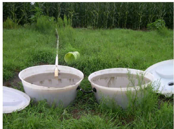
Fig. 1 Runoff tanks for collecting water samples after each runoff event
