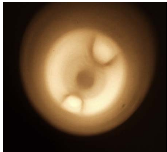
Fig. 1 Photograph of the light spot produced by the Fieldspec ® Pro near-infrared (NIR) spectroradiometer, showing that it is spatially uneven
