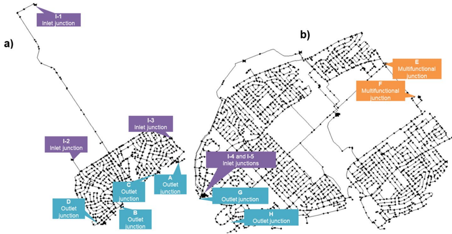
Fig. 1 EPANET models of a) Zone A and b) Zone B
