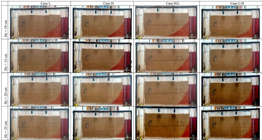
Fig. A-4 Experimental results of saltwater intrusion wedge for \theta = 90^\circ , for various aquifer cases a Case L, b Case H, c case H/L, and d Case L/H, for four various presented cutoff-wall depths
