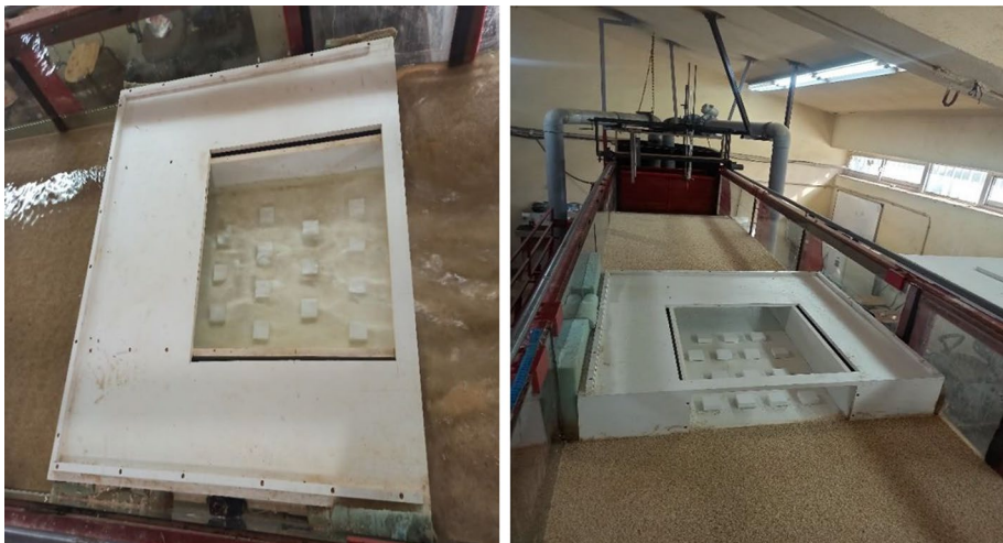
Fig. 2 Illustration of artificial roughness inside the culvert
