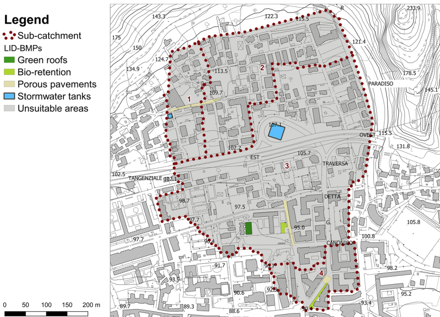
Fig. 11 Areas converted into LID-BMPs and location of stormwater detention tank of Sub-Catchment 3
