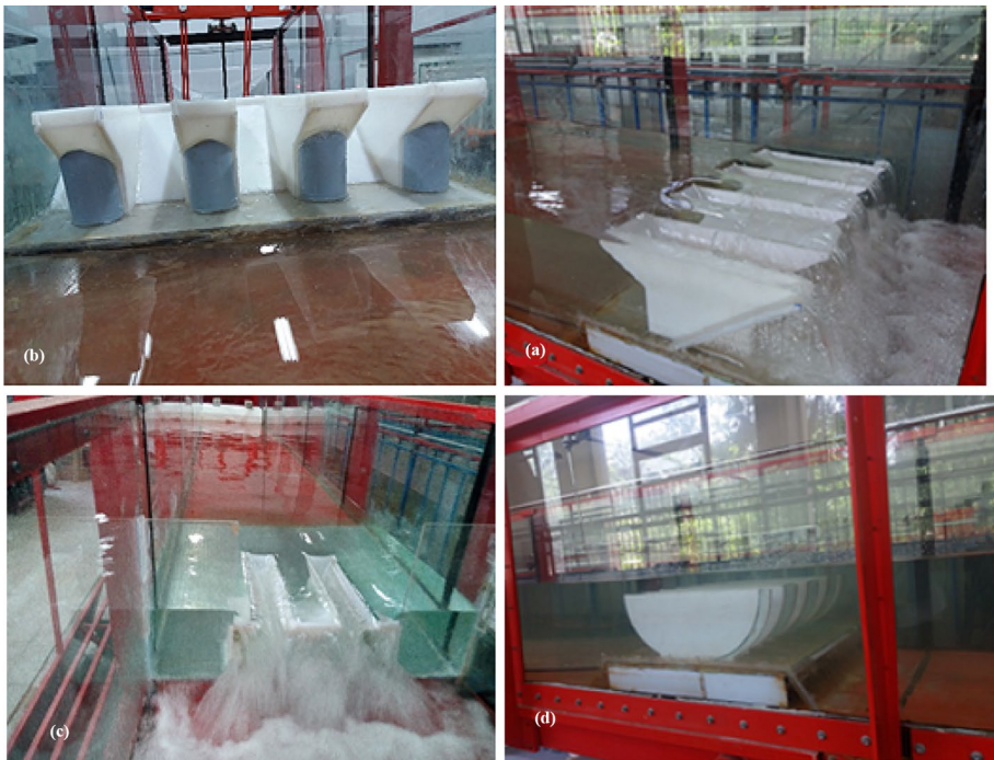
Fig. 6 (a) PK weir, (b) modified Pk weir, (c) submerged flow PK 1.25 , (d) submerged flow PKC1
