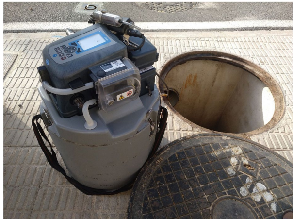
Fig. 7 Example of automatic sampler used for monitoring
