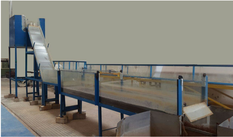
Fig. 2 The physical model of Javeh RCC dam built on hydraulic structures laboratory of Kerman University
