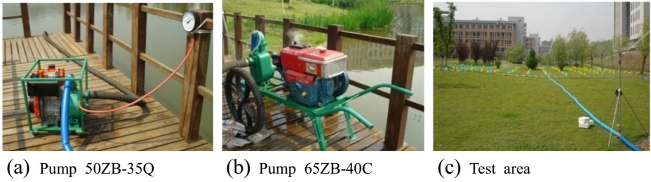
Fig. 3 Self-priming pumps and the test area (a) Pump 50ZB-35Q; (b) Pump 65ZB-40C; (c) Test area
