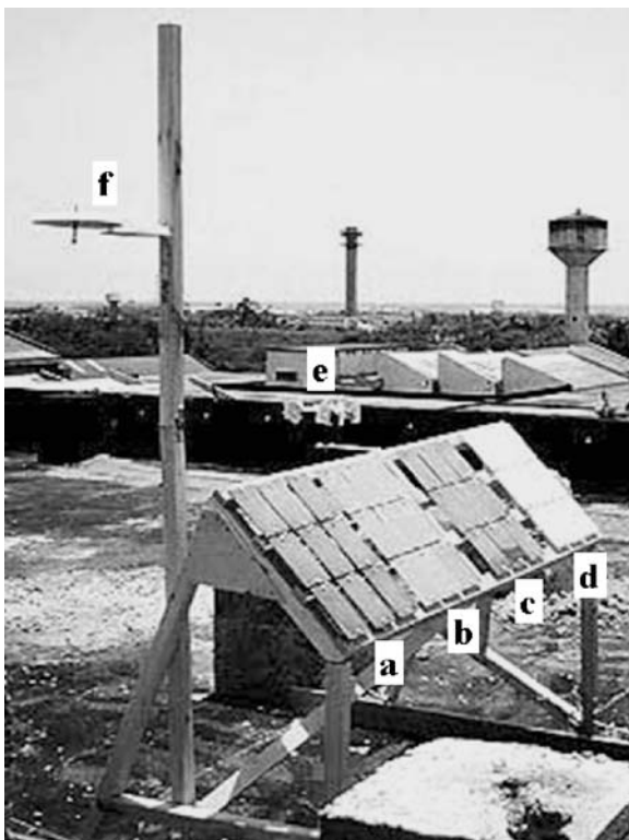
Fig. 1 Rack erected at a roof of a building in the urban site in Bhubaneswar: a carbon steel samples; b zinc samples; c copper samples; d painted steel samples; e limestone samples on a carousel; f passive samplers for gases and particulates fastened under circular discs for rain protection
