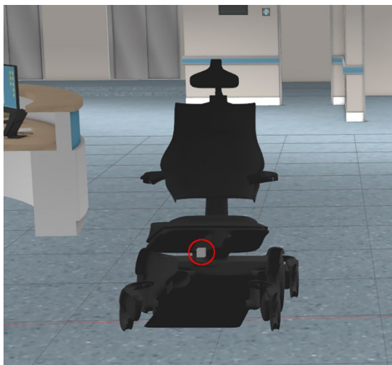
Figure 9 A detailed model of the wheelchair. The red circle highlights the RGBD sensor mounted on the wheelchair.
