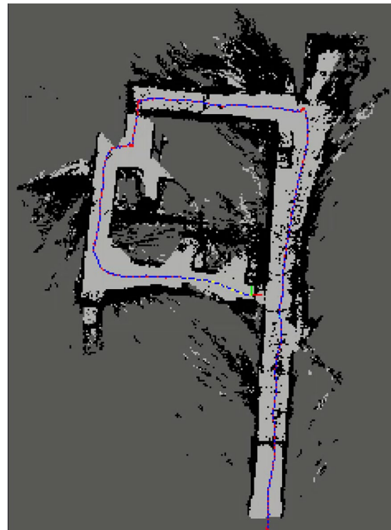
Figure 15 The wheelchair localizes itself in the mapped environment using the stereo camera data also taking its orientation into account.
