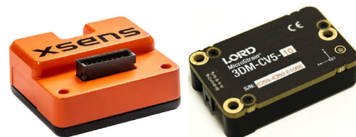
Figure 3 Commercial attitude and heading reference systems with built-in IMUs from XSens Technologies BV and LORD MicroStrain, with three accelerometers, three gyroscopes, three magnetometers and three temperature sensors for sensor calibration. These IMUs include coning and sculling compensation (see Section 5), which enables them to deliver attitude data at low rates without losing accuracy.
