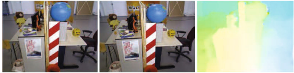
Figure 6 Two consecutive RGB frames and the output of the optical flow algorithm.
