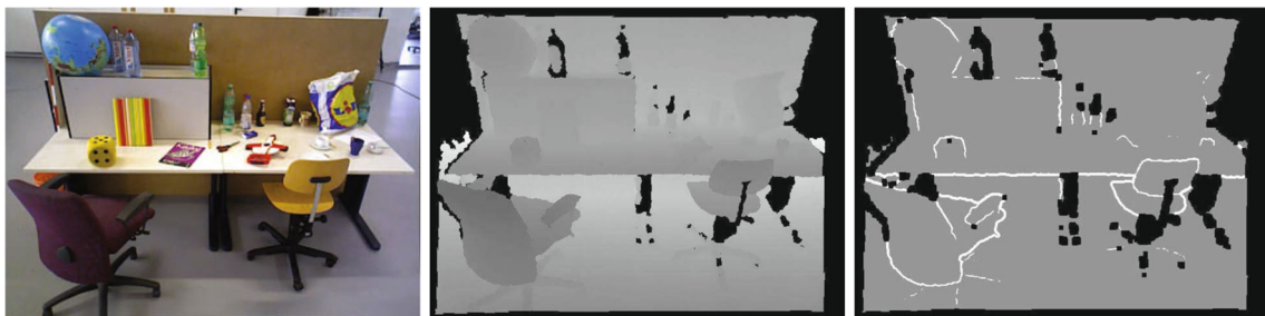
Figure 3 Example RGB, depth and classification frames from the training data generation procedure. In the classification frame gray signifies no edge, occlusion edges are white and black is for no or unreliable data.
