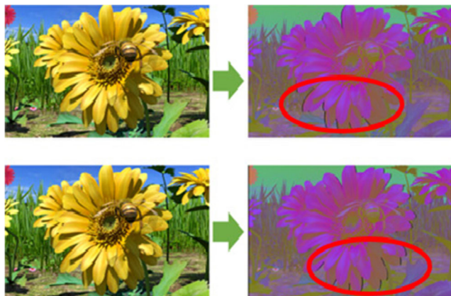
Figure 2 Hole appearance on left and right synthesized images.
