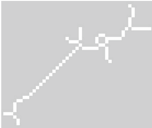
Figure 11 Result of the redundant pixel removal algorithm [16]. No gaps are present in the resulting structure skeleton (compare to Fig. 6b).
